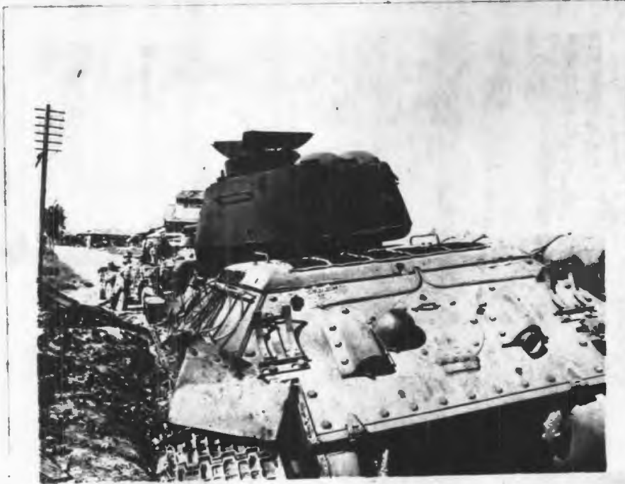
Figure 43. T34 disabled by 76-mm penetration in rear, PYONGTAEK, 27 September 1950. H. H. Braunstein
